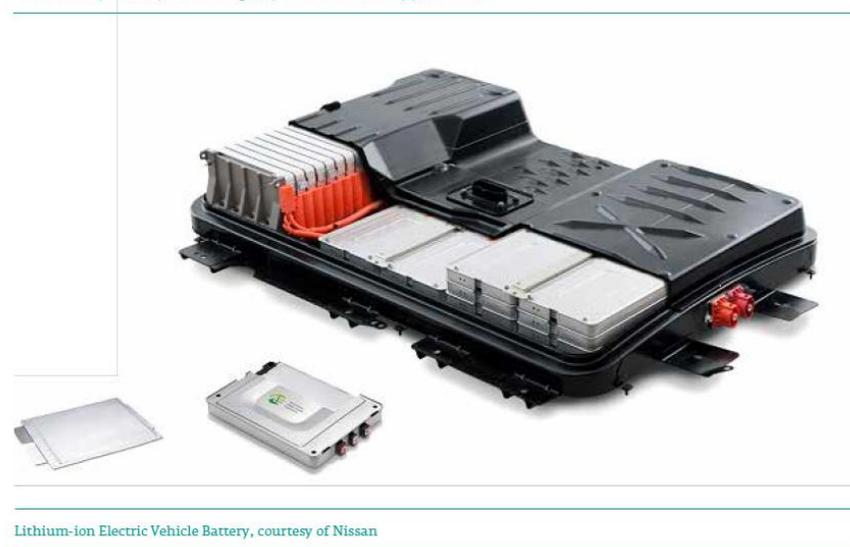
Lithium-ion Electric Vehicle Battery, courtesy of Nissan
