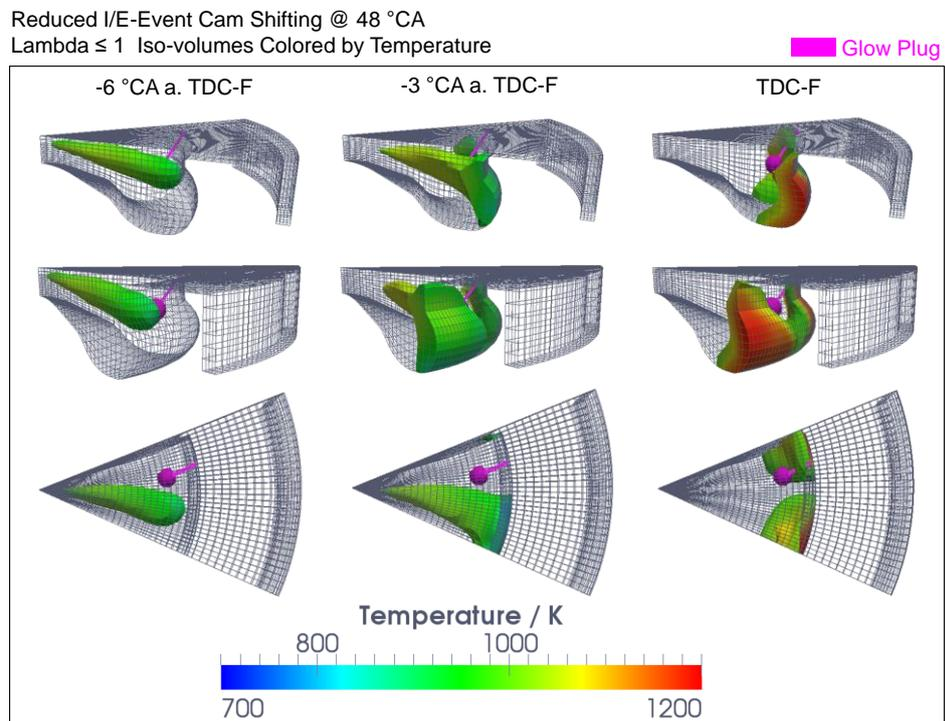
With accurate positioning of the glow plug, the modelling results have shown that a favourable interaction between the fuel spray and glow plug is possible with the chosen nozzle cone angle of 153°. For the VVT variants examined here, wider fuel
