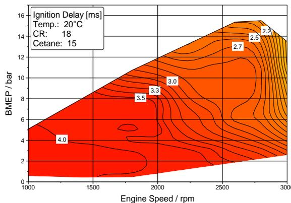
It was clear, therefore, that some form of combustion assistance (e.g. glow plug or spark plug) would be needed to support combustion under cold engine conditions and perhaps also at light loads even with a warmed-up engine. Other options to more rapidly warm-up the engine might also be beneficial, such as by-passing the intercooler and EGR cooler.
