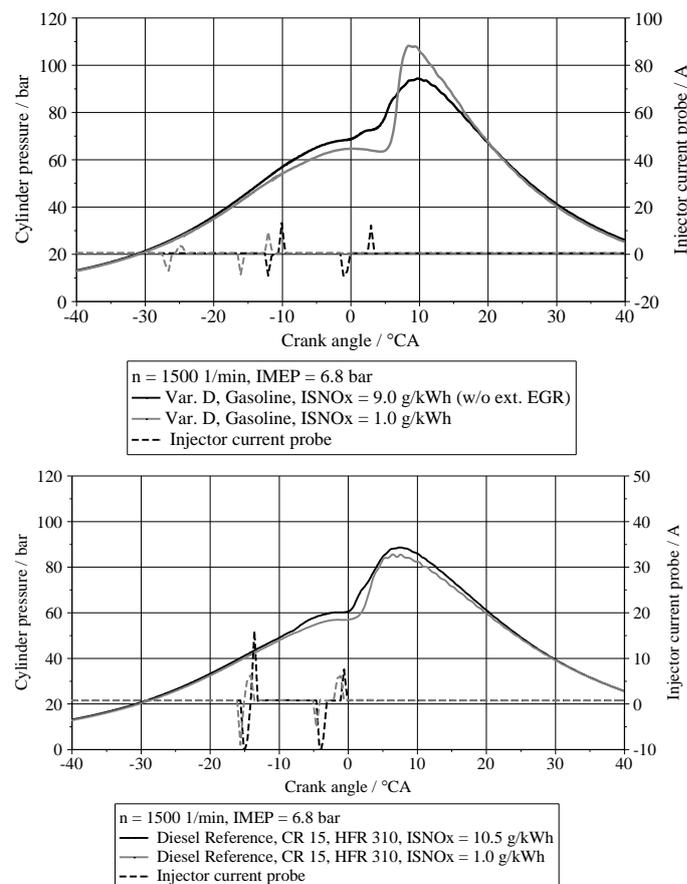
To address these limitations, a revised injection strategy was used to phase the introduction of the fuel into the cylinder. Early attempts with a split main injection
