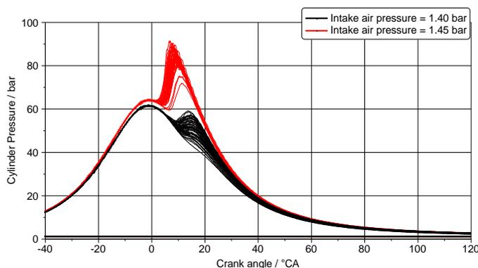
The stability or repeatability of combustion is therefore an important metric that has been used to evaluate performance throughout this study.
