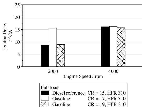
Contrary to the expectations from the paper study, the lower HFR 310 nozzles (with smaller nozzle holes) were found to perform better than the HFR 520 nozzles. Using the HFR 520 nozzles at CR 17, the maximum cylinder pressure varied dramatically at 2000 rpm so that full load could not be achieved.
