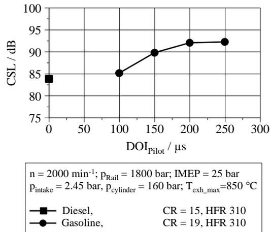
Using the pilot injection, reducing fuel injection pressure from 1800 bar to 1400 bar did not reduce noise and smoke emissions increased. For this reason, it was concluded that pilot injection at higher fuel injection pressure was the most effective strategy. With this approach, engine operation was found to be within the boundaries of 850°C maximum exhaust temperature and 160 bar peak cylinder pressure, while matching the power achieved by the diesel engine (**Figure 8**).
