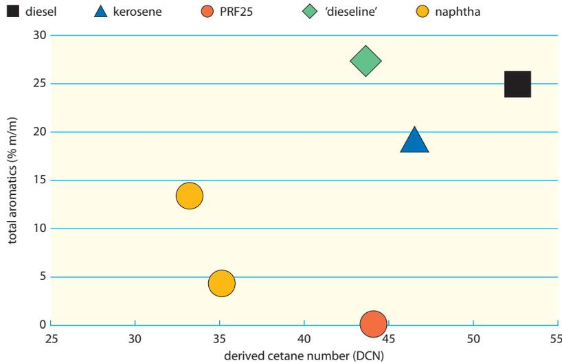
fleet of advanced combustion vehicles. The fuels included both conventional and experimental blends. In addition to a typical European diesel fuel and commercial kerosene, a 'dieseline' blend of diesel and gasoline fuels and two naphtha fuels sampled from refinery process units were tested. A Primary Reference Fuel (PRF25), blended from pure chemicals boiling in the gasoline range, was also tested.
