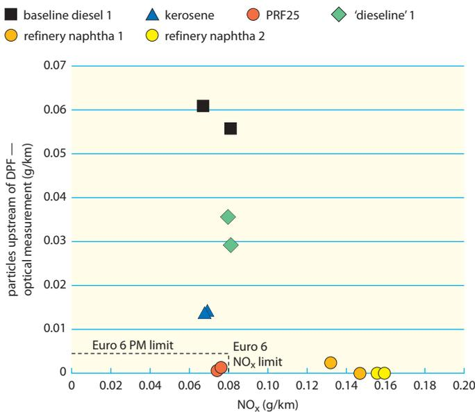
**Figure 3b Tailpipe NO<sub>x</sub> versus PM emissions over the NEDC**
