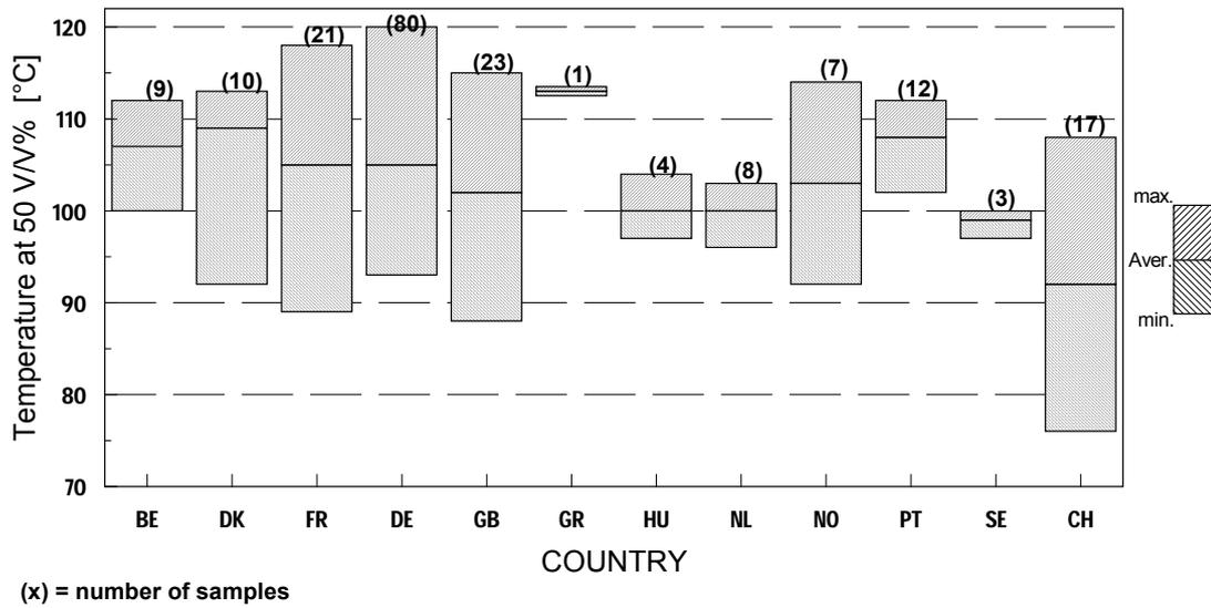
**Figure 8** Distillation characteristics of super unleaded (95)
