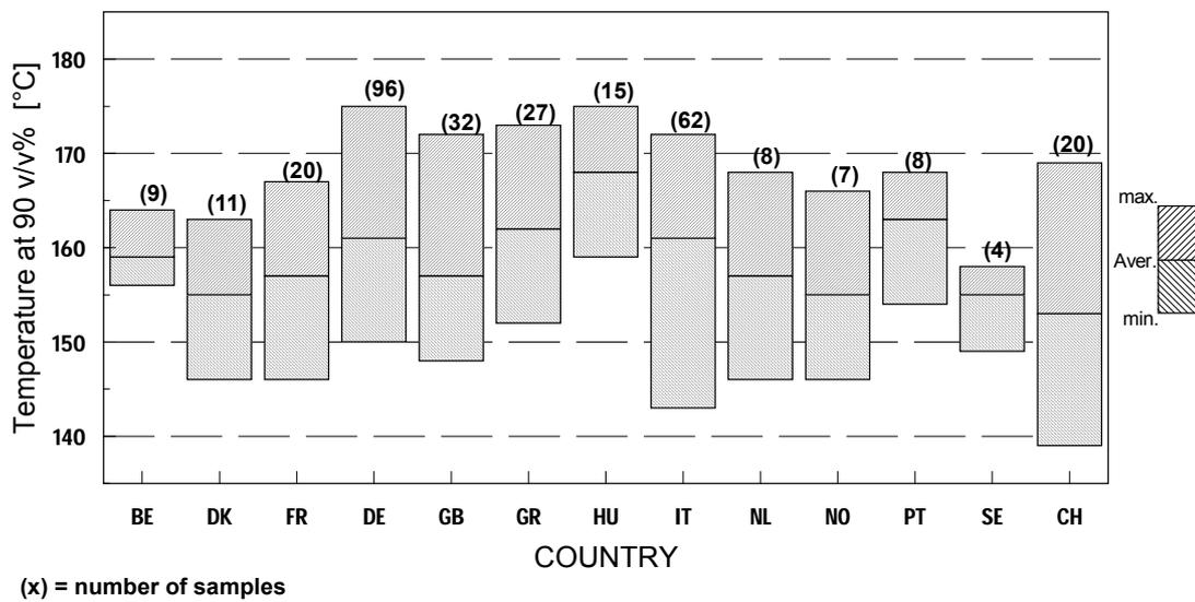
**Figure 9** Distillation characteristics of super unleaded (98)
