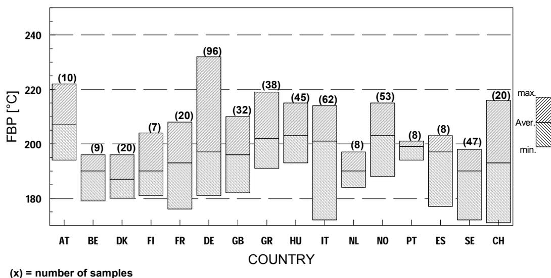
**Figure 11** Distillation characteristics of super unleaded (98)
