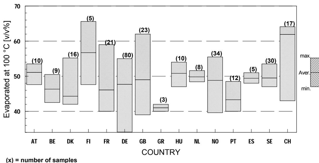
**Figure 16** Distillation characteristics of super unleaded (95)
