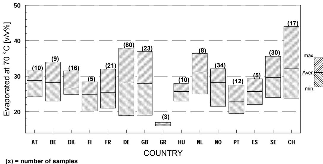
**Figure 14** Distillation characteristics of super unleaded (95)
