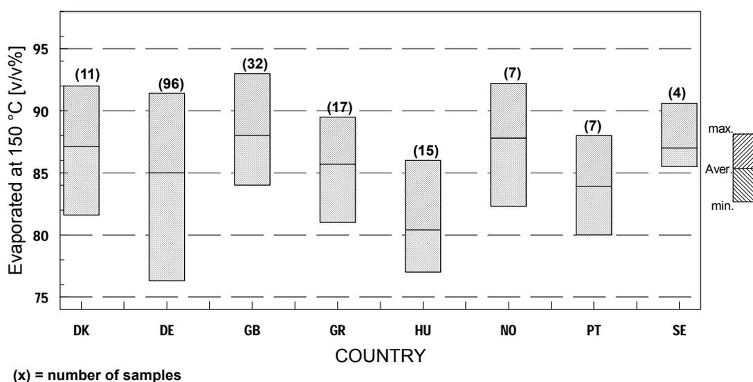
**Figure 17** Distillation characteristics of super unleaded (98)
