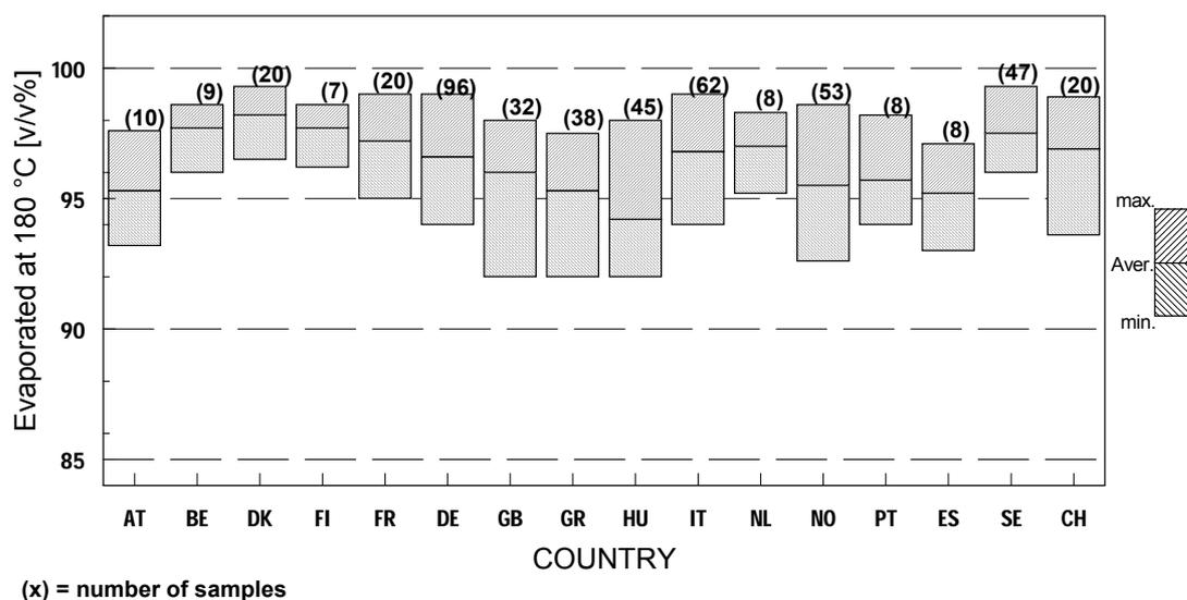
**Figure 19** Distillation characteristics of super unleaded (98)
