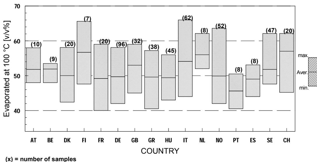
**Figure 15** Distillation characteristics of super unleaded (98)
