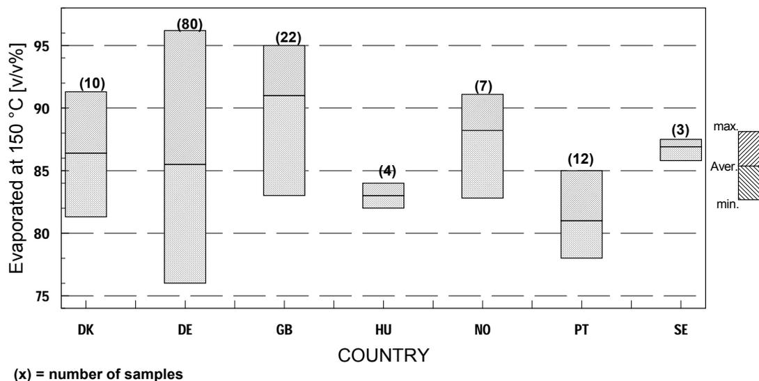
**Figure 18** Distillation characteristics of super unleaded (95)
