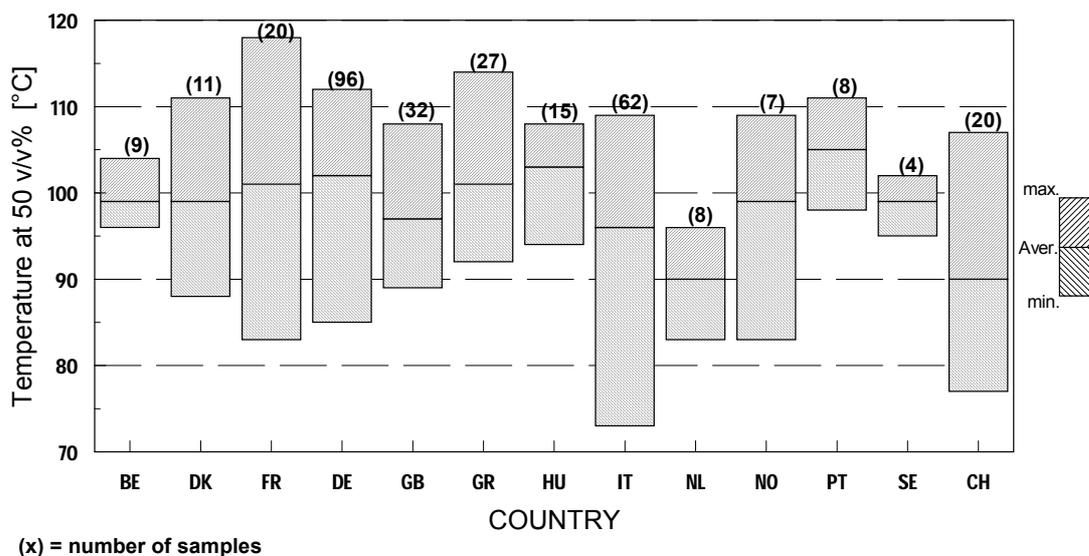
**Figure 7** Distillation characteristics of super unleaded (98)
