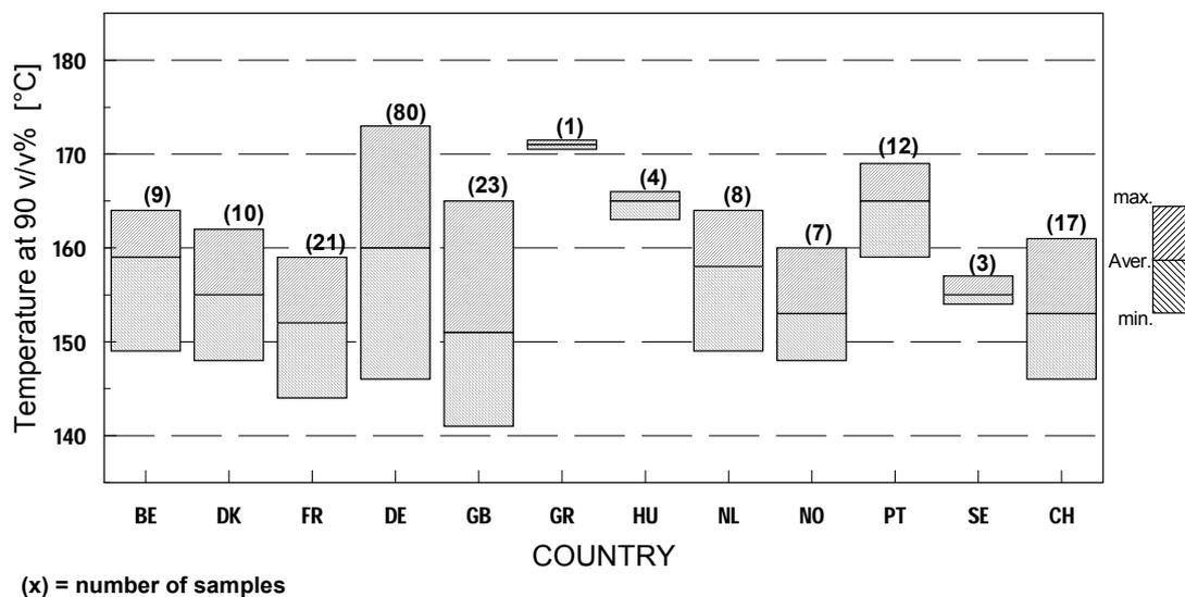
**Figure 10** Distillation characteristics of super unleaded (95)
