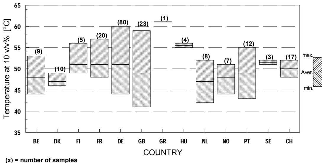
**Figure 6** Distillation characteristics of super unleaded (95)
