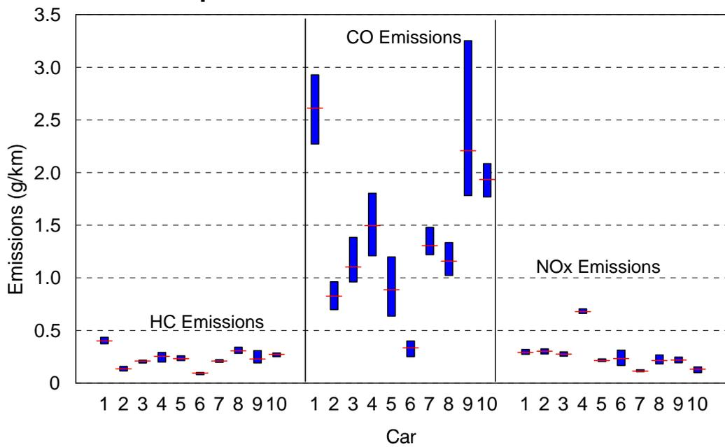
The variation across the fuels for each car is represented by the vertical bars. The horizontal line indicates the mean emissions for each car averaged over the seven fuels. The ten cars are represented for each emissions species across the horizontal axis
