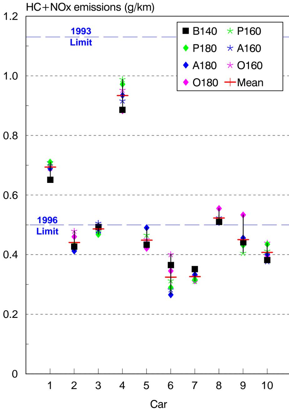
The asterisks and crosses show the emissions for each of the seven fuels in each car. The red + shows the mean emissions for each car over the seven fuels.
