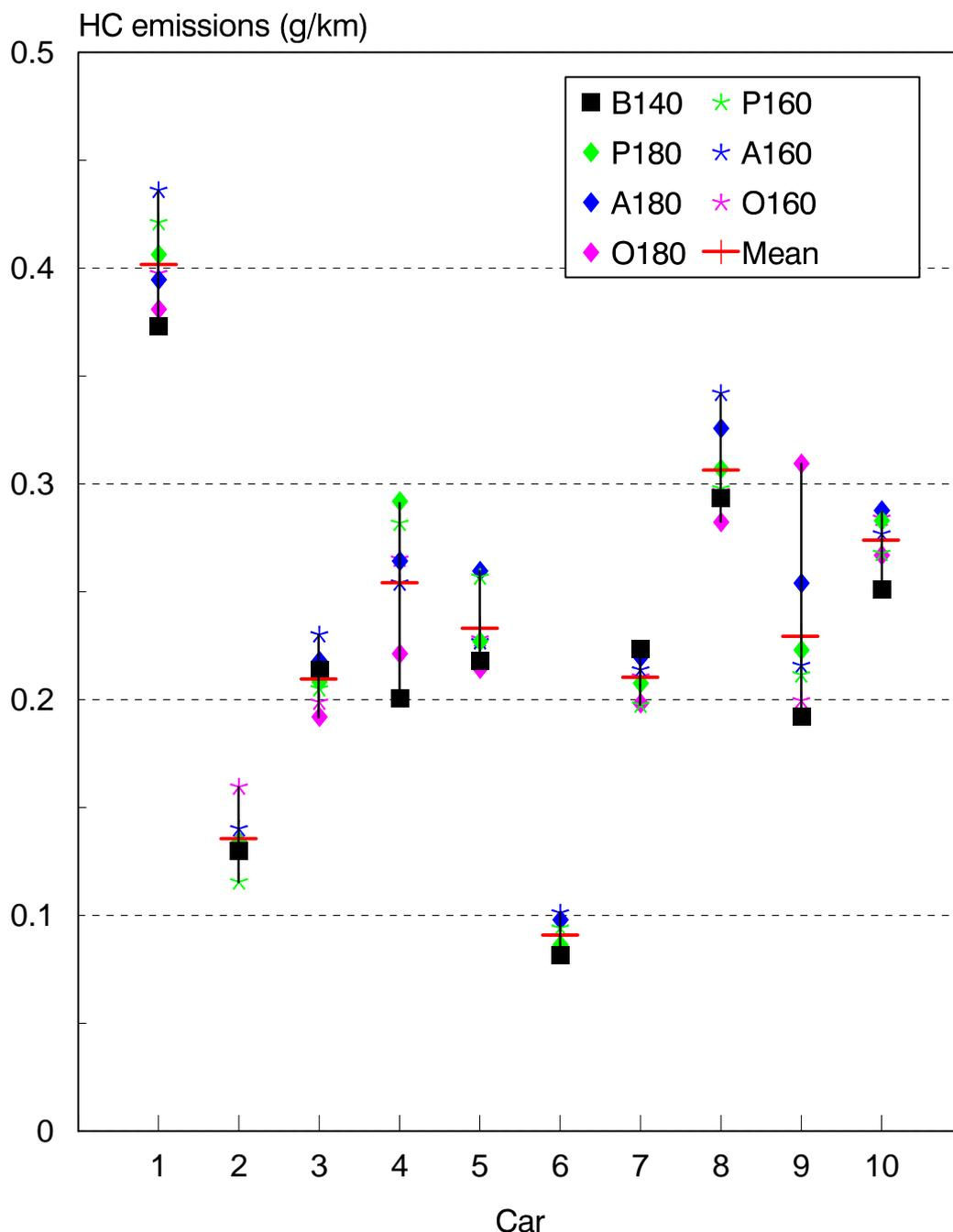
The asterisks and crosses show the emissions for each of the seven fuels in each car. The red + shows the mean emissions for each car over the seven fuels.
