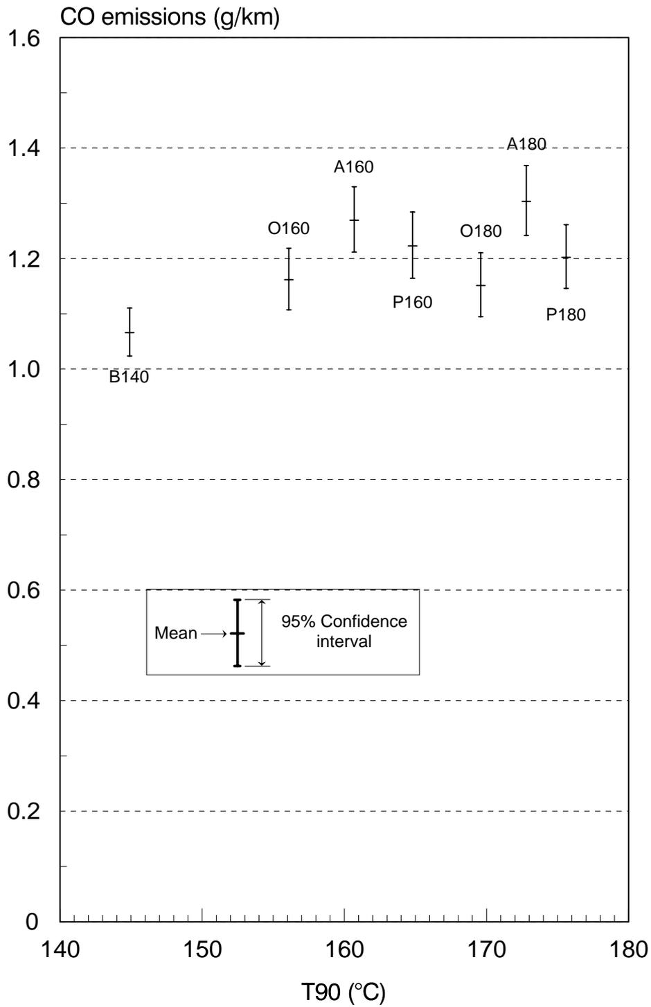
**Figure 9** Total cycle CO Emissions (Ten-car Geometric Mean)
