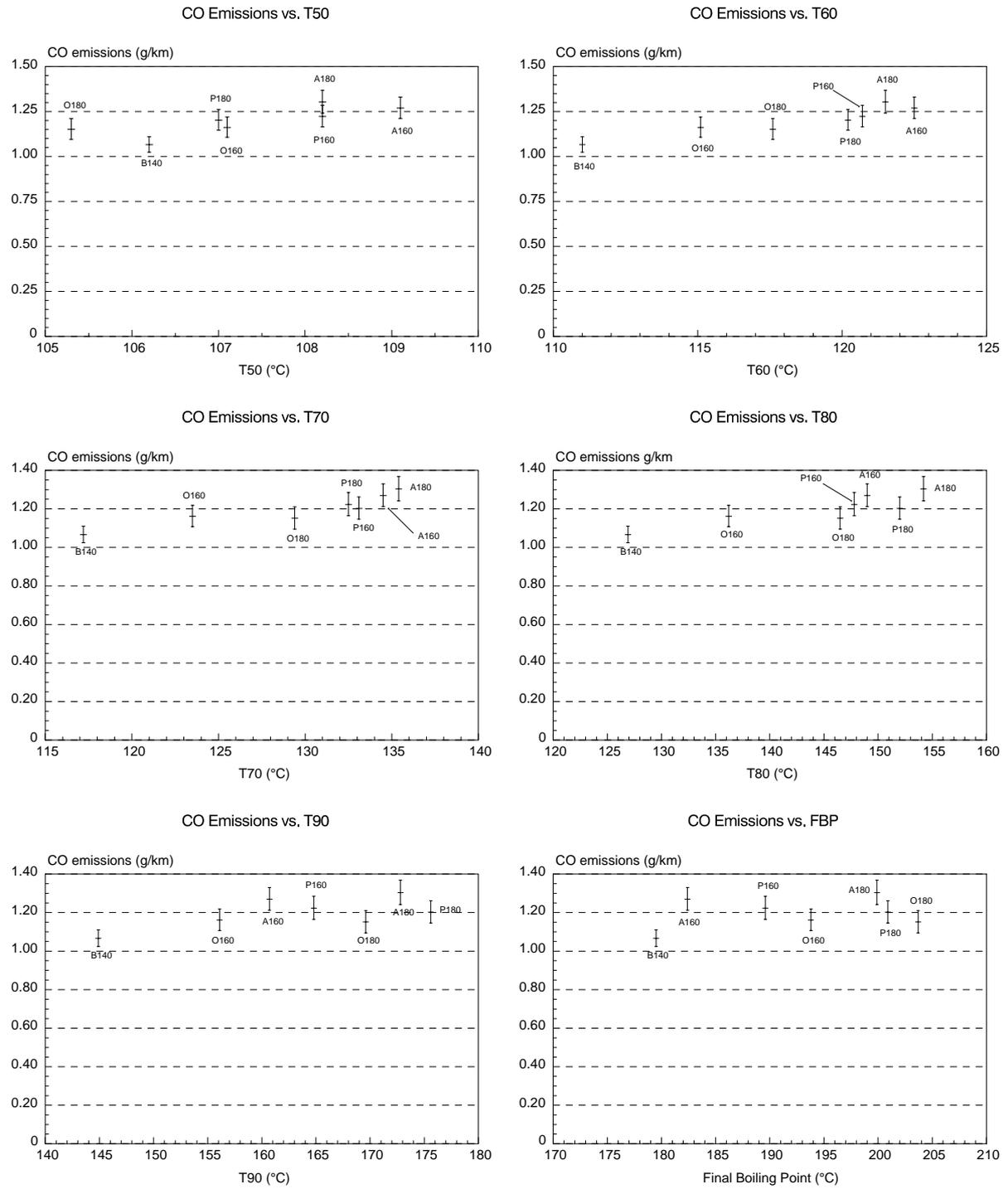
**Figure D** Total Cycle CO Emissions
