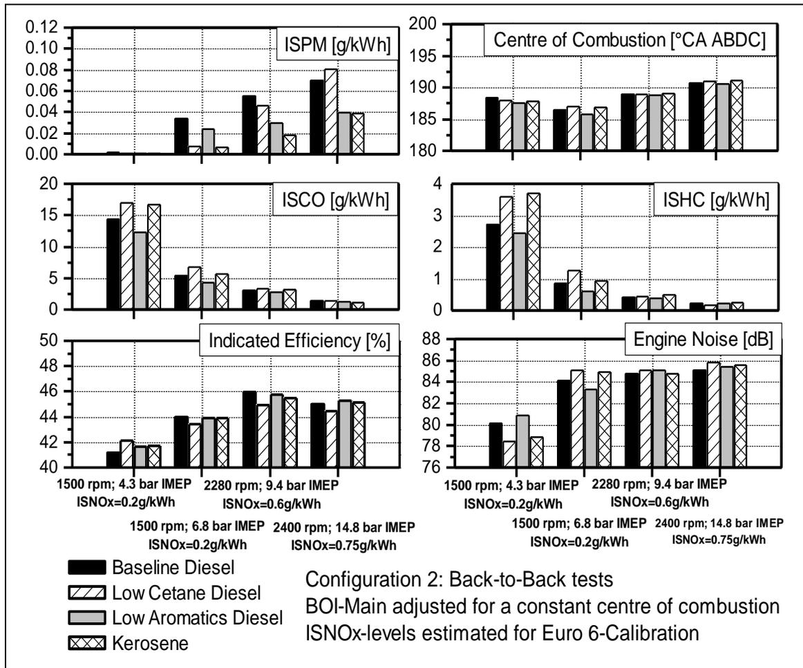
The NOx levels for each test point were those required to meet Euro 6 limits, as indicated in **Table 5**. The centre of combustion was adjusted to be the same for each fuel.
