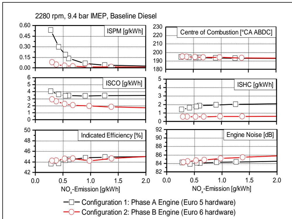
At the 2280 rpm, 9.4 bar IMEP part-load point, there was only a small change in the centre of combustion. For this reason, the indicated efficiency also stayed at about the same level. The Phase B engine had much lower emissions at this part-load point. The PM, CO, and HC emissions were all significantly lower although there was a slight increase in noise emissions.
