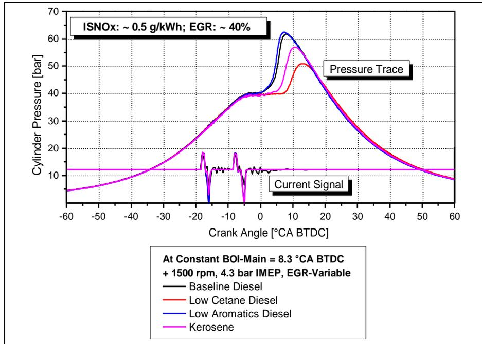
**Figure 10** Pressure traces at 1500 rpm, 4.3 bar IMEP in the Phase B engine with injection timings adjusted to achieve a constant centre of combustion
