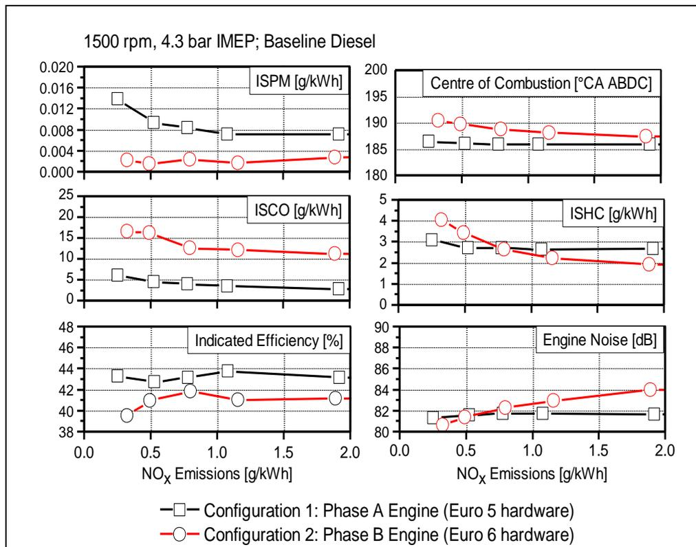
At the 1500 rpm, 4.3 bar IMEP part-load point, lowering the Compression Ratio from 16 in the Phase A engine to 15 in the Phase B engine resulted in a later (retarded) centre of combustion. As expected, this later centre of combustion led to a lower indicated efficiency and increased the CO emissions by a factor of 3. This increase could be problematic for the oxidation catalyst because of the low exhaust gas
