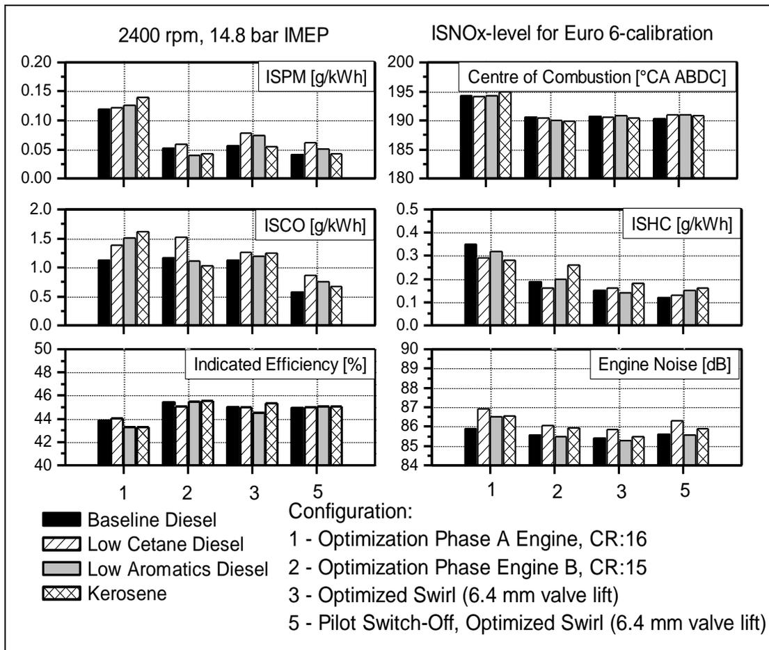
The engine improvements from the Phase A engine to the Phase B engine dramatically reduced the PM emissions at all part-load points. The fuel effects and the variations of the centre of combustion were different at different loads and none of the fuels was clearly the best at all test conditions.
