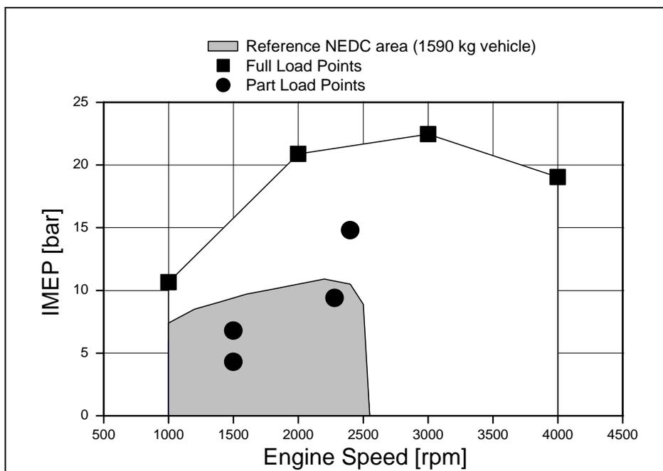
At the start of this study, it was decided to investigate three part-load points. A fourth lower part-load point at 1500 rpm, 6.8 bar was added later at the start of testing on the Phase B engine.
