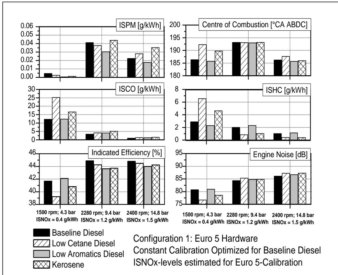
The NOx levels at each test point were those required to meet Euro 5 emissions limits, as indicated in **Table 5**. Because the injection timing was fixed in these tests, the centre of combustion varied between fuels.
