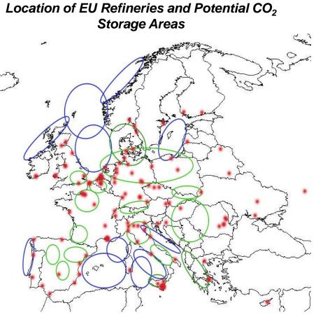
**Source**: The European Technology Platform for Zero Emission Fossil Fuel Power Plants (ZEP) **Legend**: Red dots are refineries, blue and green bounded areas are potential offshore and onshore storage areas
