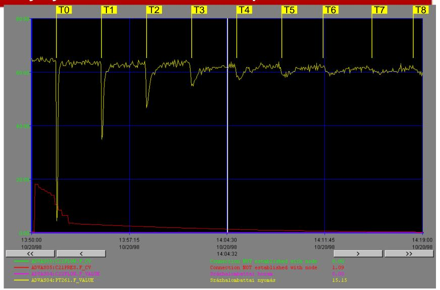
Pressure waves can be detected after 2000 Km propagation along the pipeline
