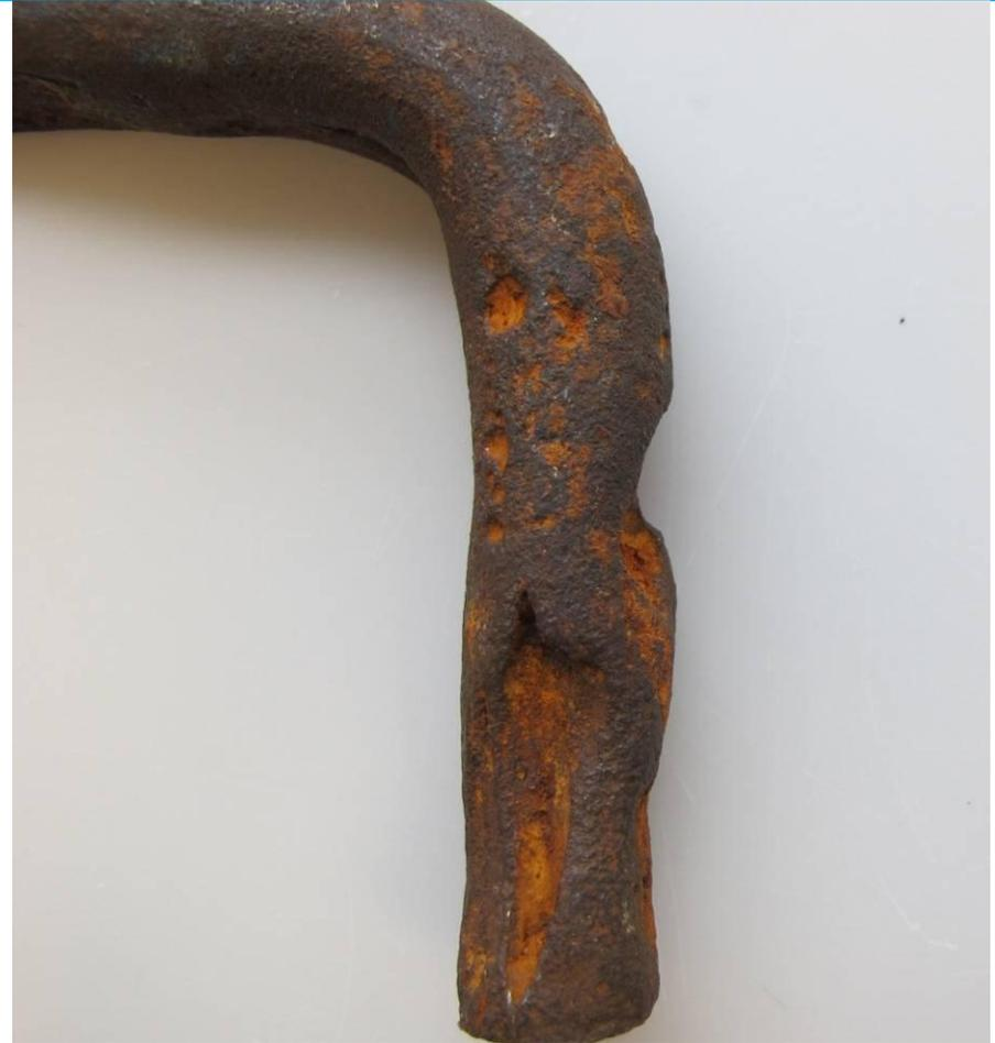
Evidence of srb corrosion
