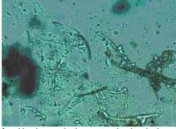
fungi hyphes and micro water droplets in the fuel phase,ca. 800x
