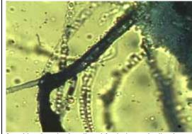
fungi hyphes in the diesel fuel phase (yellow), extend into water phase (dark), ca. 800x
