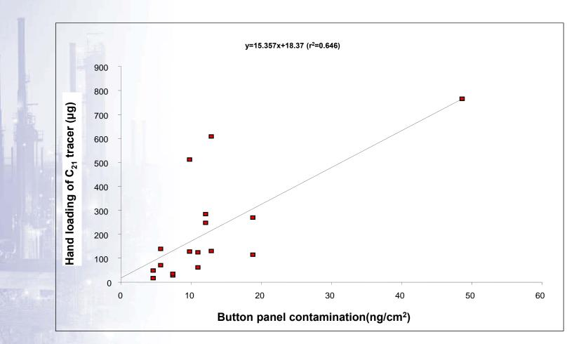
Linear regression analysis comparing C<sub>21</sub> contamination on the button panel with loading onto the hands
